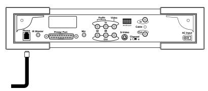
Connect the telephone cord to the Phone jack on the back of the Internet Terminal and to your home's telephone jack.
